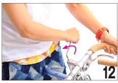
Loosen the stem bolt with a 6mm allen wrench. Only loosen it between a half and full turn (180-360 degrees).
