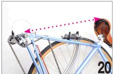
Imagine a line from the rear derailleur to the back of the saddle. This will be the plane (ground plane) that the bike rests on once it is properly bundled. Nothing should extend beyond it.
