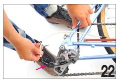
The rear derailleur housing is slid away from the derailleur. This allows the bundle to rest on the ground plane with out damaging the derailleur, or affecting it's adjustment. Refer to the picture on the cover if this is unclear.
