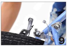
If your straddle wire is still attached to one side of your brakes, unhook the yoke from the straddle wire.
