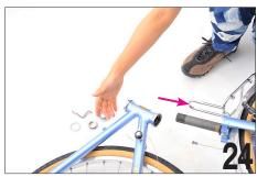
Remove all of the headset parts including the cable hanger from the steer tube (fork).
