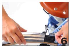
Remove the wing nut on the rear fender.
