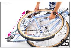
Place the front wheel with the fork still attached on top of the frame
