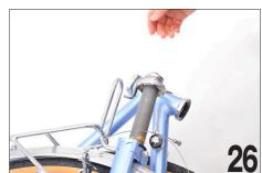
Make sure to re-install all of the headset hardware including the cable hanger to prevent all those parts from getting lost during your trip.
