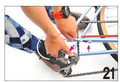
With the shifter in the highest gear (most difficult to pedal) push the derailleur towards the center of the bike. While holding it in this position remove the cable housing from the stop.
