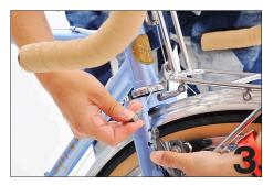
Unhook the straddle cable from the brake arm. Some brakes allow this on both arms. Others have the starddle bolted to the other arm.
