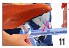
The stops are slotted to allow the inner wire to come free.
