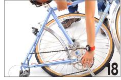
Lay the frame down on top of the rear wheel as shown. Note that the the cassette/freewheel is facing the ground.
