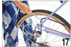
Use an allen key to place the chain on the chain rest on the inside of the seat stay. This will help keep your hands
