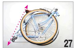
Note the alignment of the fork and front rack with the frame.
