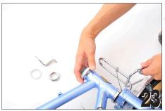
Use a 32mm wrench to loosen the headset locknut.
