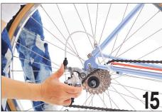
Pull the derailleur rearward to allow the wheel to drop free from the rear end.
